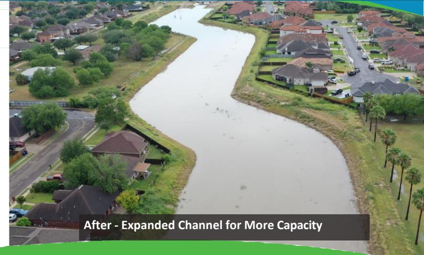
After - Expanded Channel for More Capacity
